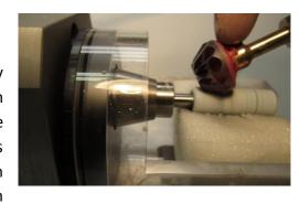
facet. That keeps grooves from forming like they would if the stone were held in one place. The difference in concave faceting is the polishing mandrel oscillates back and forth and the stone is held in one place in most production model concave faceting machines.
