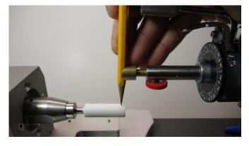
on. Let the pencil mark the mandrel for several oscillating motions of the machine. The result will show you what your machine is doing to the concave facet. One of the most important features of the Fantasy or Concave Machine by Ultra Tec is the ability to adjust the ratio of RPM per oscillation. Beginning at the pre-polish stage the lines should cross at a sharp angle as the machine travels in and out. This is what eliminates the striated lines and gives a true
