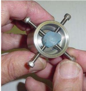
Set the rough into position - manipulate the floor position and the four Adjusting Screws to grip the gem rough. "Eyeball" it into position. The fine adjustment will happen later.
