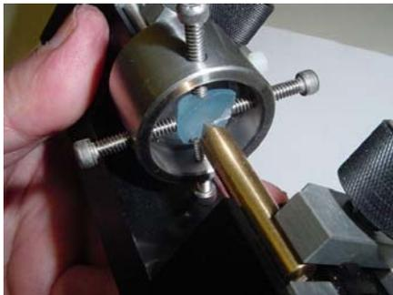
Set the loaded Guiu Dopper into one side of your Transfer Fixture. Set the Centerpoint Guide into the other side of your Transfer fixture.
