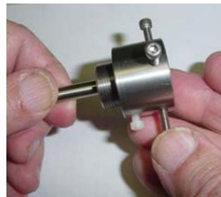
You will see that the outer Barrel can be rotated (you may have to loosen the nylon screw - it is only hand tight). The affect of that Barrel rotation is to raise or lower the “floor” - the bottom support for the gem rough.
