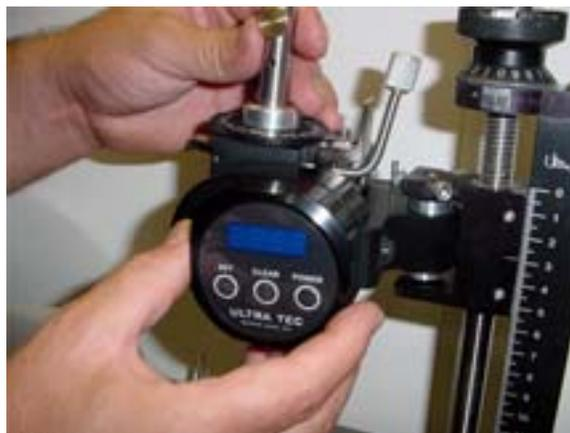
3.3 Holding the DAD to the Yoke with your left hand, with the Spindle still pointing UP, slightly tighten the set screw nearest the Mast (don't make it tight—that comes later)—as shown in the first picture below. Then, continuing to hold the DAD to the Yoke, slightly tighten the forward set screw (again, don't make it tight—that comes later).
