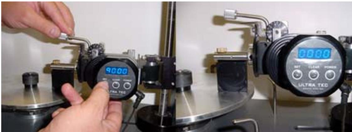
(whoops—did you press it more than once? Start over—back to 4.3—pull the plug—replug and proceed. raise up—lower—confirm that the Spindle is flat against the Block-- **press the SET button ONCE**).
