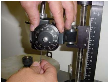
Before you set it aside, look at it and see how the clamping action of the set screws held it to the Yoke—the DAD is going to assemble to the Yoke in the same way. Set it aside (know where you put it—it serves as a hope-you-never-use “spare tire”).
