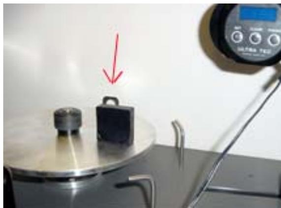
4.4.2 With the Angle Stop loose, lower the vertical position—approaching the 90 degrees (represented by the top surface of the Calibration Block)--it's OK to "ride it down", resting on the Block, as shown (the display is still flashing 90.00—it's prompting you to set the 90 degree position). Gradually lower...lower...THERE.
