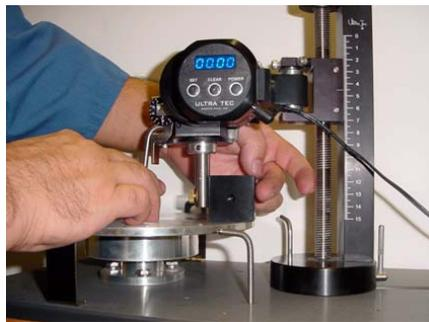
You will now go through a 0-setting procedure that's pretty much the same as the prior 90 degree procedure—except, with gravity no longer helping, it will be watching the gap...watching...watching...adjusting with the Fine Adjusting Knob...until the light showing through the gap is pinched off. It's there at 0 degrees.
