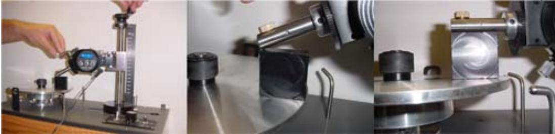
How do you KNOW it's "there"? As you lower the position, and the Spindle is evening out against the top surface of the Calibration Block, you watched as the gap closed ... closed...slowly closed...adjusting with the Vertical Knob--seeing what light comes through the gap. When the light is pinched-off—it's THERE. 90 degrees.
