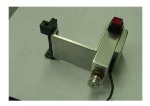
The Bracket "Adder" is added to the Bracket—then it clamps slips onto the Main Bearing Block where it is gripped by tightening the set screws in the bottom arm—a "C-clamp" type of gripping.
