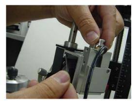
2.2 Mount the driven Pulley onto the Quill. To do that, remove the Dop Retention Knob, so that the Pulley slides past that point, push the Pulley flush to the Index gear Hub, and tighten the set screw that holds the Pulley in position. Re-insert the Dop Retention Knob.
