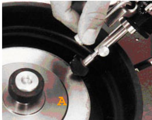
**NOTE:** If you accidentally drop your adapter, be sure that surface **A** (underside of flange) is not damaged. That surface is precision machined for flatness and perpendicularity to the center hole preventing any wobble of the saw. If you should nick the surface, removing any raised material with a stone or fine file will restore its accuracy.
